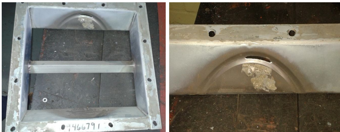
Figure 10.1: The eroded metal guide replaced at Nova Foods with different coatings
