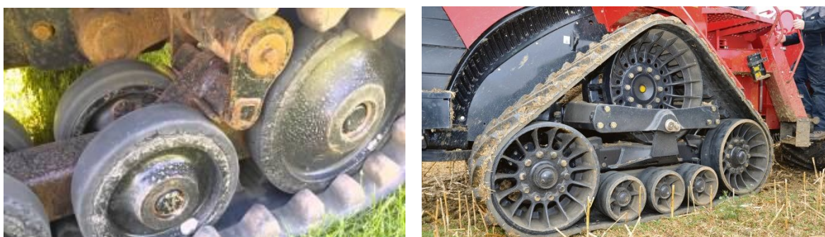
Figure 2.2: Roller bearings on tracks that are used in place of tyres on tractors with high horsepower (Tracklayers, n.d.)
