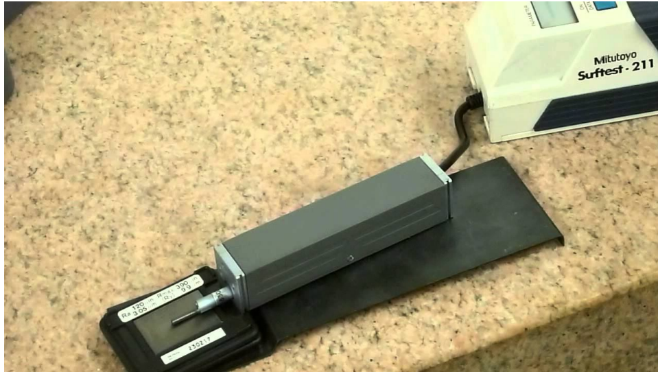
Figure 8.6: The Mitutoyo Surftest: 211 surface roughness tester (Portable Surface Roughness Tester, 2014)
