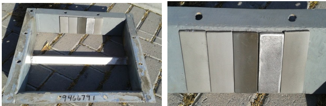
Figure 10.2: Five different coatings on the different plates mounted to the grain guide ready for installation
