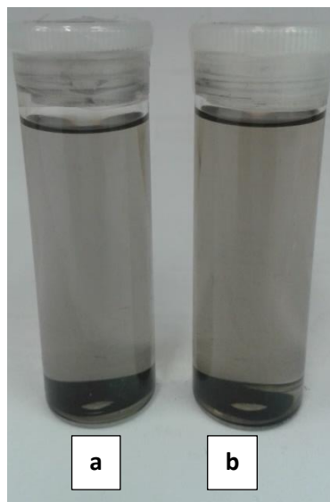
Figure 4.22: Solvation analysis by visual representation of a) polymer deprived solution and b) multi-functional compatibilizing polymer containing solution with EG.
