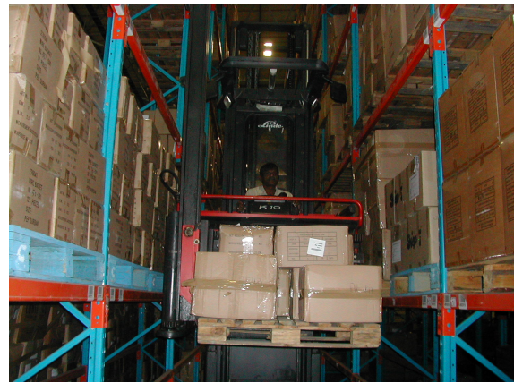
(b) A photograph of a loaded high-lift lifting a pallet in the storage racks.
