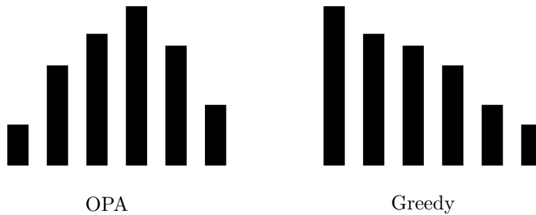
Figure 3.4: A schematic representation of the layouts for both the OPA and GS heuristics. The height of each bar represents the probability that an order will require a SKU for carousel systems or the actual number of orders requiring that SKU in the case of the picking line under consideration.
