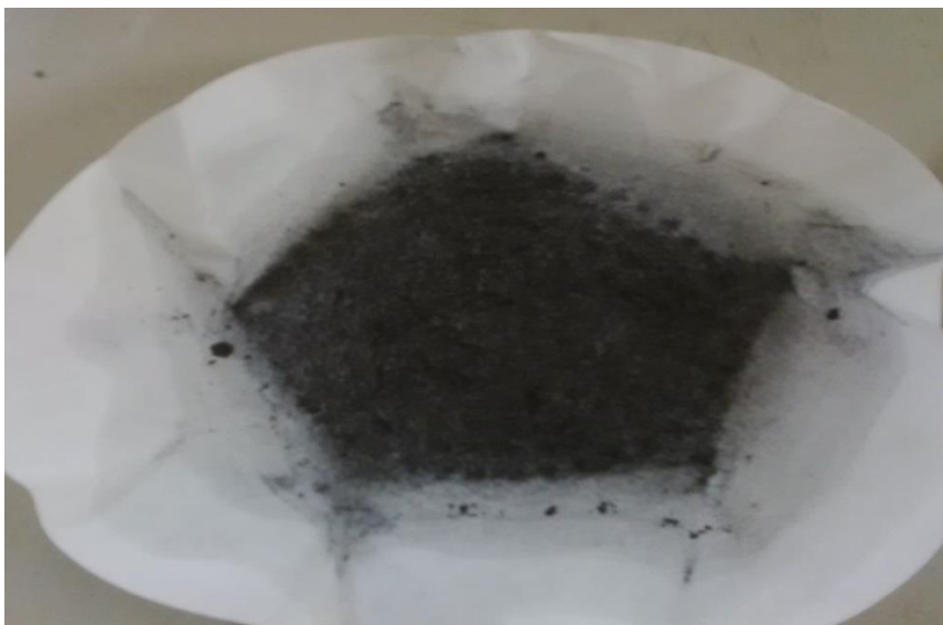
Figure 4.23: The effect of agitation speed on carbon loaded with Au. Dark portions indicate the amount of carbon fines obtained from carbon granules at the agitation speed of 1200rev/min (Pre-treatment conditions: 1200 rev/min, 80°C and 30 min)
