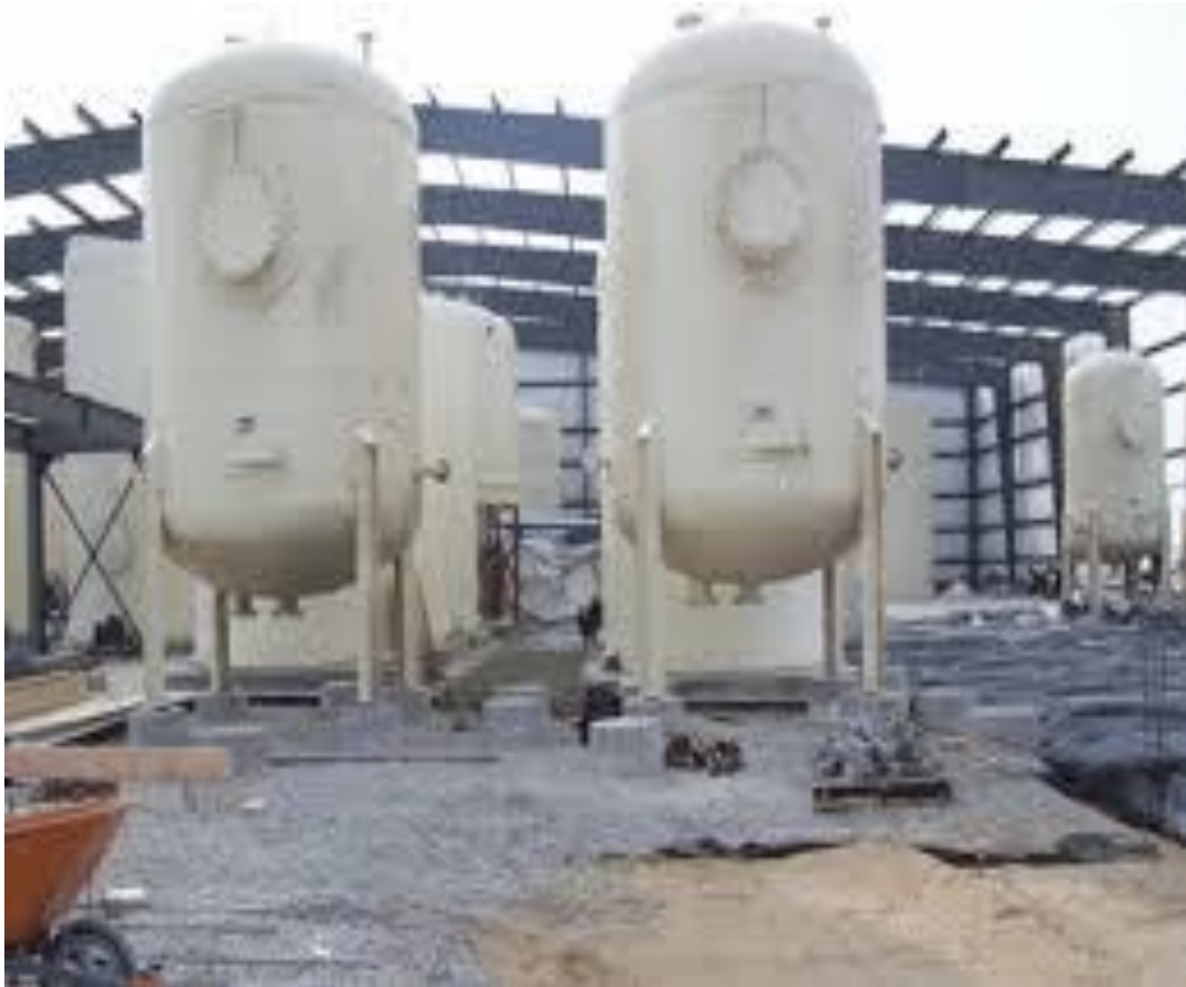
Figure 2.8 Typical Elution columns. Sourced from Ur energy (2013)
