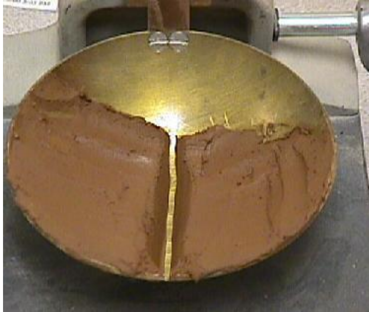
Figure 3-1: 13mm groove made in soil.
