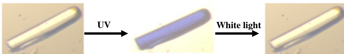
Figure 6.21 Photographic evidence of a PCCP_2 crystal undergoing a reversible colour change when exposed to visible and ultraviolet light
