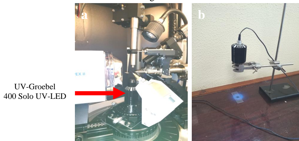
Figure 6.4 Photographs of a) continuous* and b) intermittent irradiation experimental configurations using a 365 nm UV light source.
