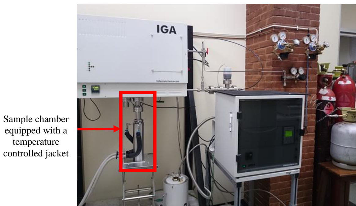
Figure 2.1 Photograph of the Intelligent Gravimetric Analyser (IGA-002) and gas cylinders.
