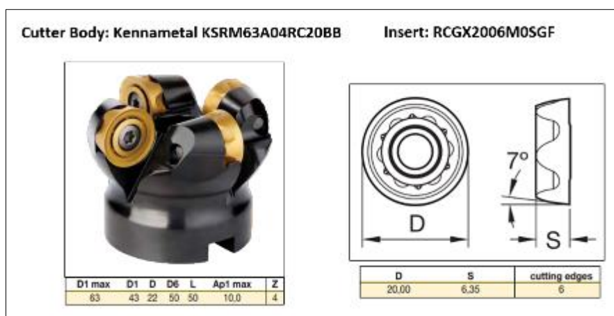
Figure 77: Kennametal Beyond Blast KSRM cutter ad RCGX round inserts
