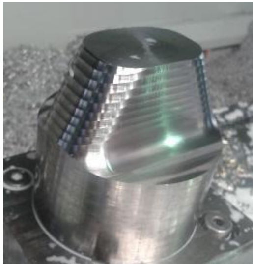
Figure 87: Helical milling path for roughing of the billet
