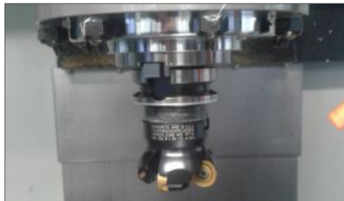
Figure 89: KSRM cutter and four new RCGX inserts on the Leadwell V-50L
