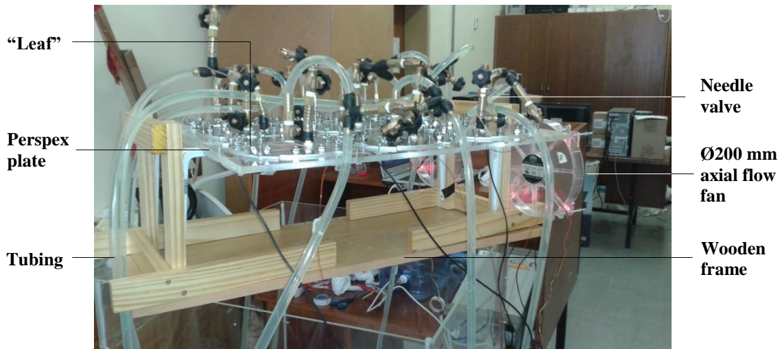
Figure 3.17: “Leaf” assembly mounted on suspended wooden frame
