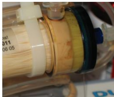
Figure A.7: Hollow fibre cartridge (FiberCellSystems. 2011. Production of Recombinant Proteins and Monoclonal Antibodies in Hollow-Fiber Bioreactors . [Online]. Available: http://www.fibercellsystems.com/documents/Article-RecombinantandMonoclonal-Cadwell.pdf . [Accessed 17 November 2014].)
