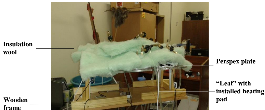
Figure 3.18: “Leaf” assembly with heat pads covered with insulation wool
