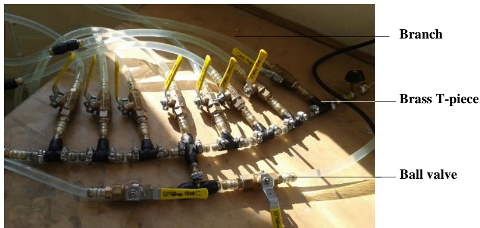
Figure 3.13: Manifold connection used in multiple branch system
