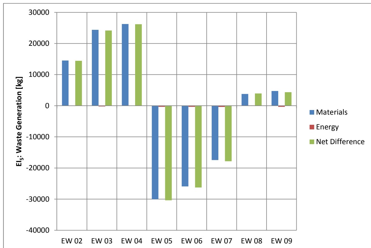
FIGURE 7-3: FULL LCA WASTE GENERATION IMPACTS IN COMPARISON WITH THE REFERENCE BUILDING
