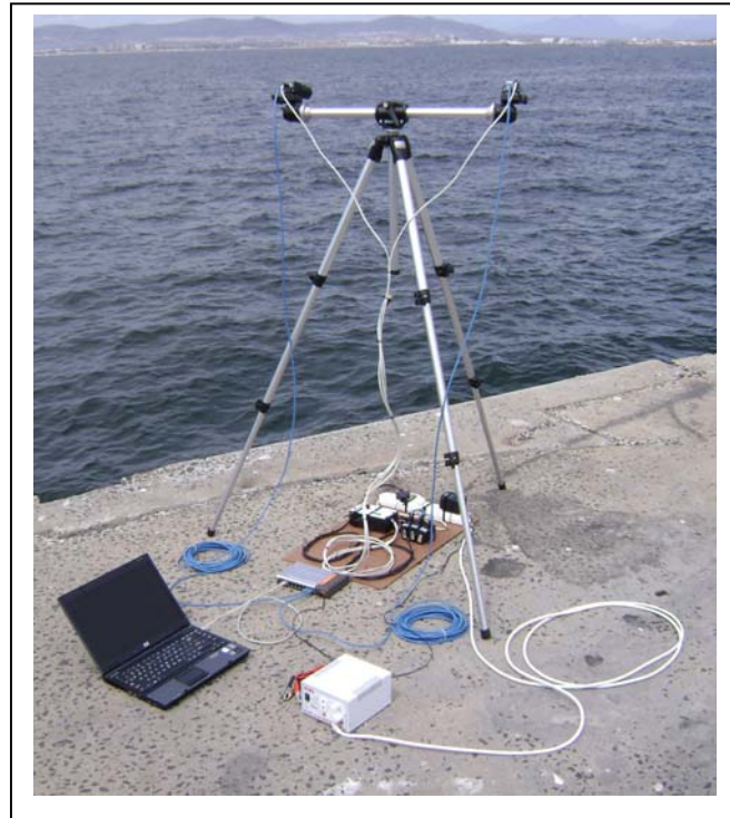
Figure 39: Typical camera set-up for capturing of stereoscopic video imagery
