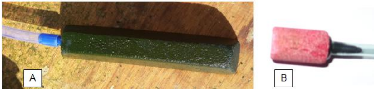
Figure 3.6: Gas dispersion units that were used during testing, A) large air stone, B) small air stone.
