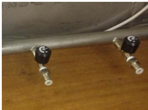
Figure 3.7: Two valves extruding from the manifold that was used to ensure a constant gas flow rate
