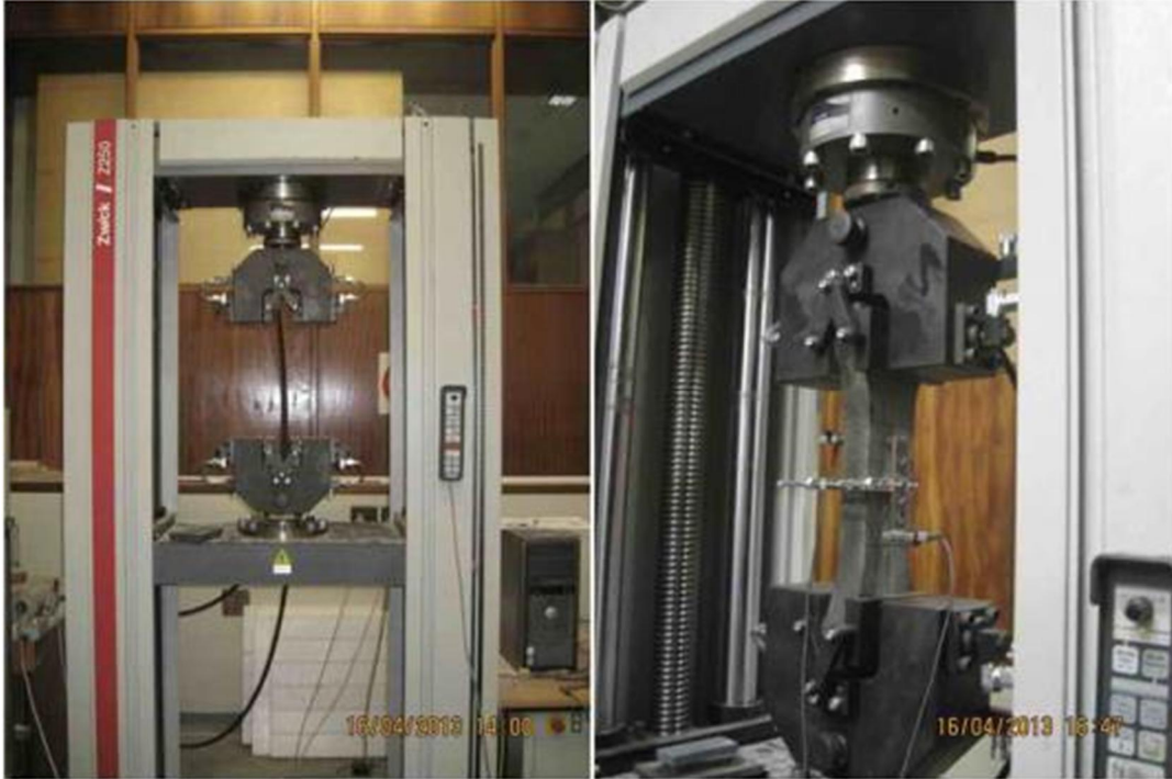
Figure 6-1: Direct tensile test setup.
