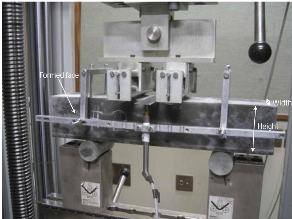
Figure 6-12: Test setup for four point flexural test.
