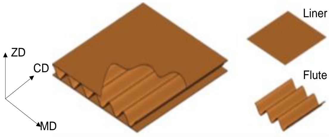
Figure 7.1: Structure of a corrugated paperboard.
