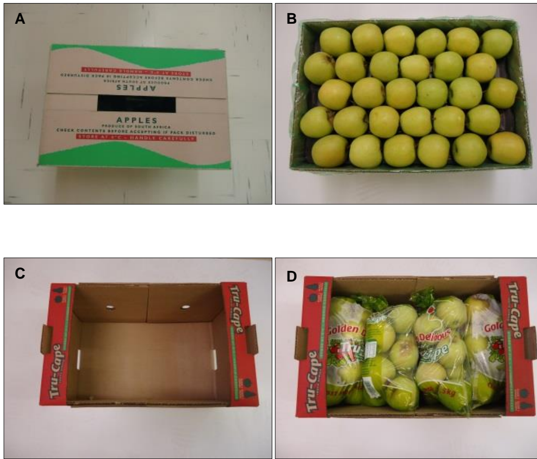
Figure 3.1: Packaging designs used: (A) MK4 box; (B) Tray arrangement in MK4 box; (C) Econo box; (D) Fruit packed in plastic bags inside Econo box.
