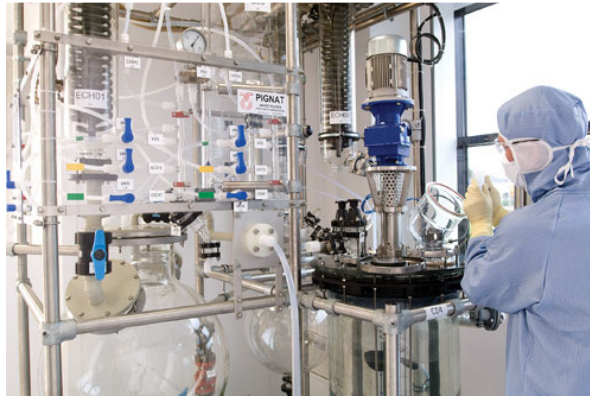
Figure 2: Peptide synthesis using liquid phase chemistry (Russell, 2012)
