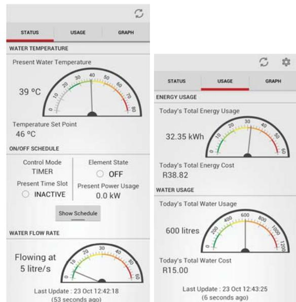
Fig. 2. Status (Left) and Usage (Right) tab of smartphone application
