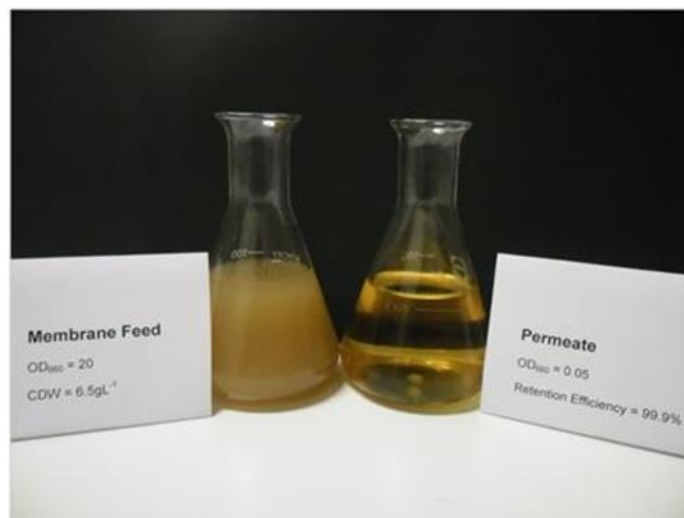
Figure 58: Optical examination of the retention efficiency of the MFU. Concentrated sample from culture mixture (left) and permeate (right)
