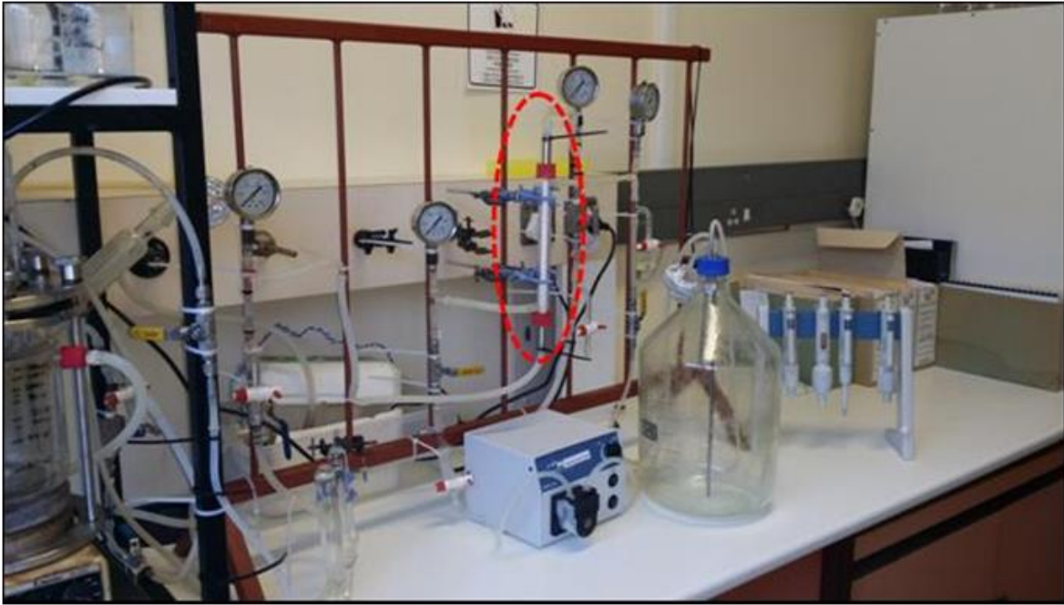
Figure 100: Single tubular membrane microfiltration unit (indicated by red ellipse), permeate reservoir, and backflush pump
