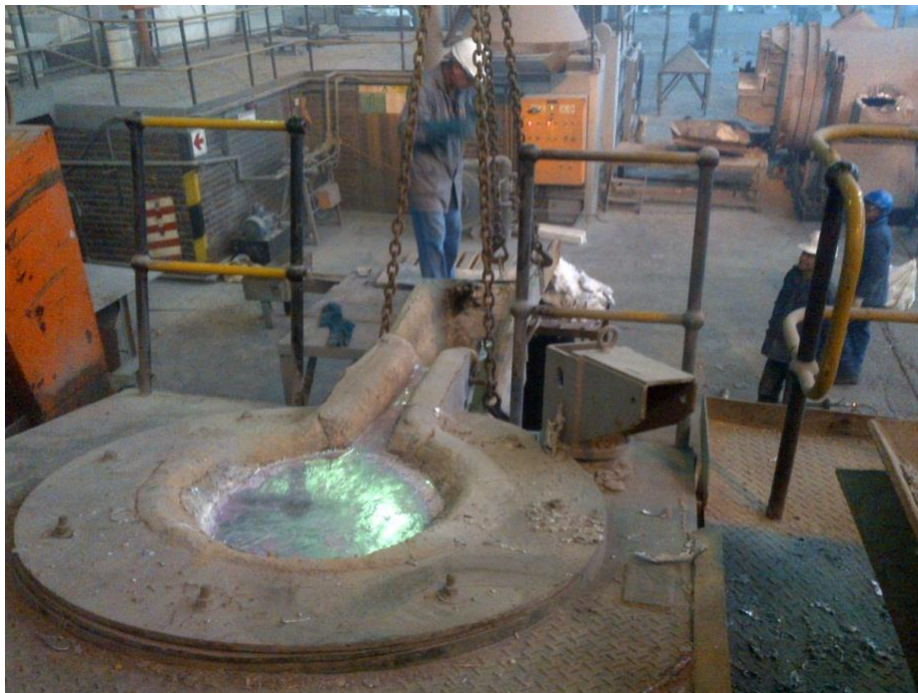
Figure 46 - Casting of AlSi12 into test section
