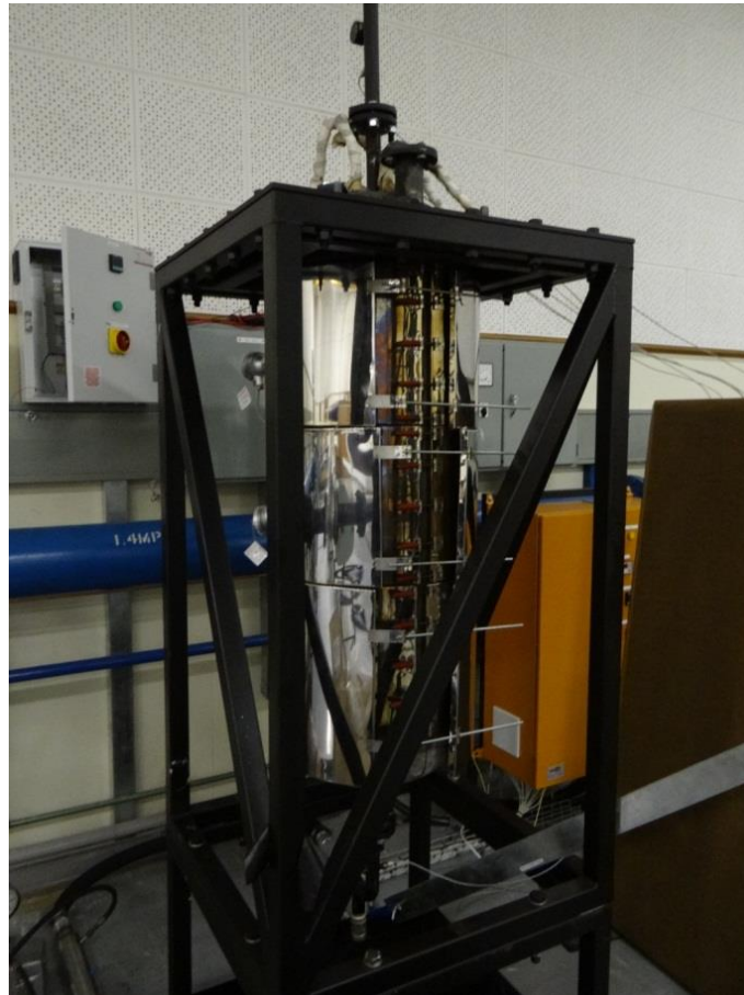
Figure 47 - Test section suspended in frame with heating elements and cladding (cladding still open)
