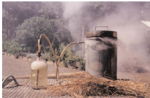
Figure 2: Apparatus for producing smoke-saturated water
