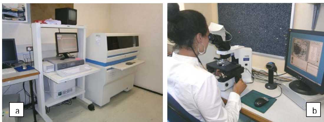
Figure 2.14: FP (a) is a computerised, automated screening device, networked to a review station (b) where FOV's are reviewed by a cytotechnologist.
