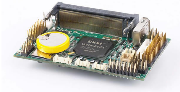
Figure 3.8: Roboard RB-100 used for the main controller (Roboard, 2012)
