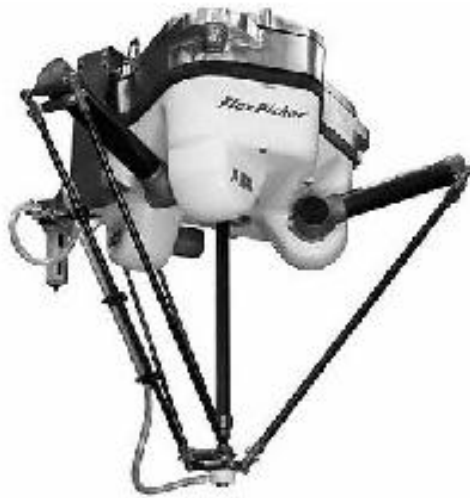
Figure 6: Industrial version of the DELTA robot, the FlexPicker IRB 340 (from ABB).
