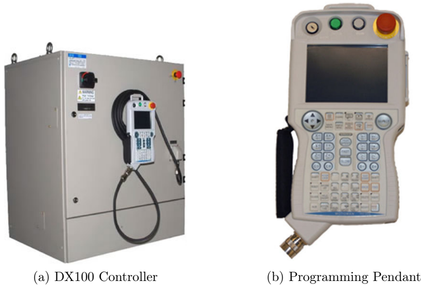
Figure 4.1.5: Basic Components of a Robotic System
