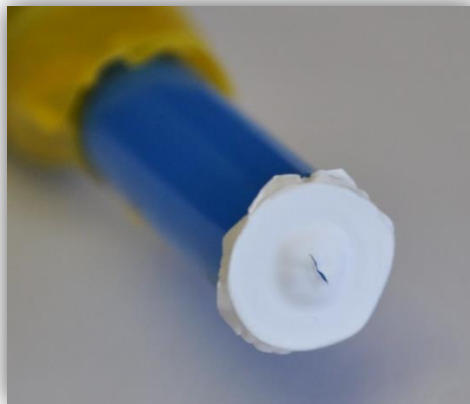
Figure 4-11: Tearing of material during in vitro tests
