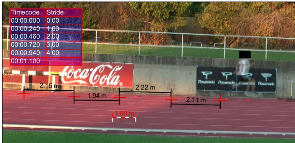
Photograph 4. The software supports electronic marking of all points of ground contact from the third stride to the 10m mark, and then calculates both stride length and stride frequency
