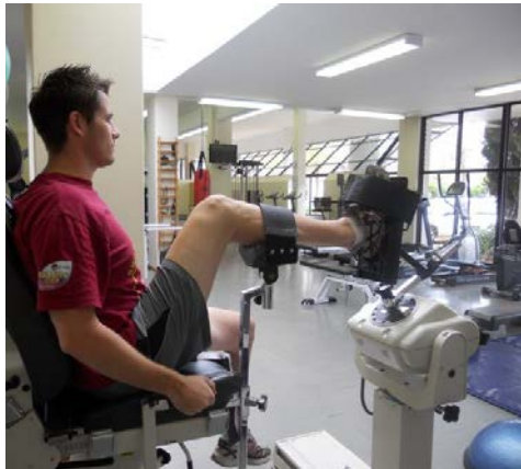
Figure 4.13. Isokinetic strength testing conducted in the inversion/eversion mode. Tests were conducted at 30 deg.sec -1 and 60 deg.sec -1 .
