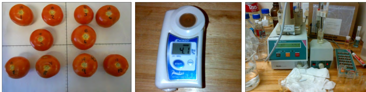
Figure 5.2: i) Representative tomatoes selected from plot 1B for quality analysis, ii) sugar content analysis (brix %) using the PAL Refractometer and iii) Titratable acidity using the titrino automatic titrator.
