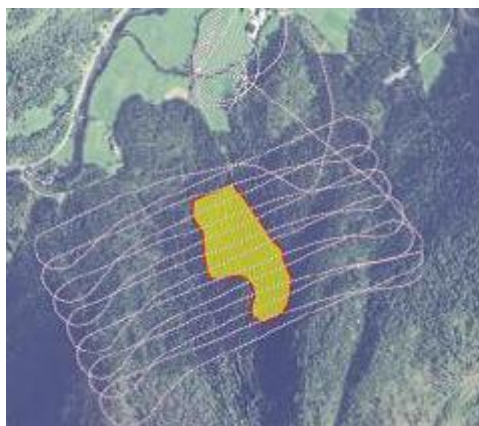
Figure 1: The flight path flown by the Gatewing aircraft – the yellow polygon represents the stand of interest.
