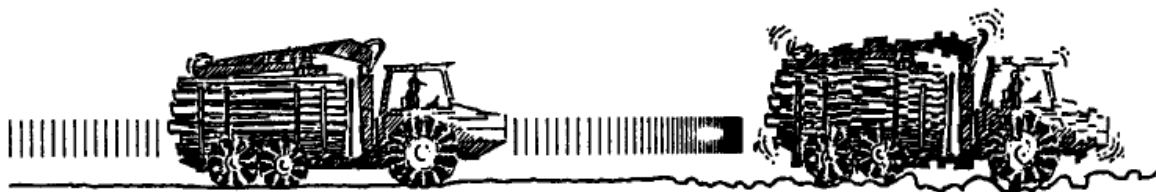
Figure 3: In addition to or in combination with pitch and roll, micro-topography also determines driving speed but is not easily obtainable from LiDAR DEMs.
