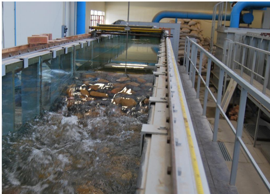
Figure 3-2: Uniform flow approaching the arrestor in the laboratory setup
