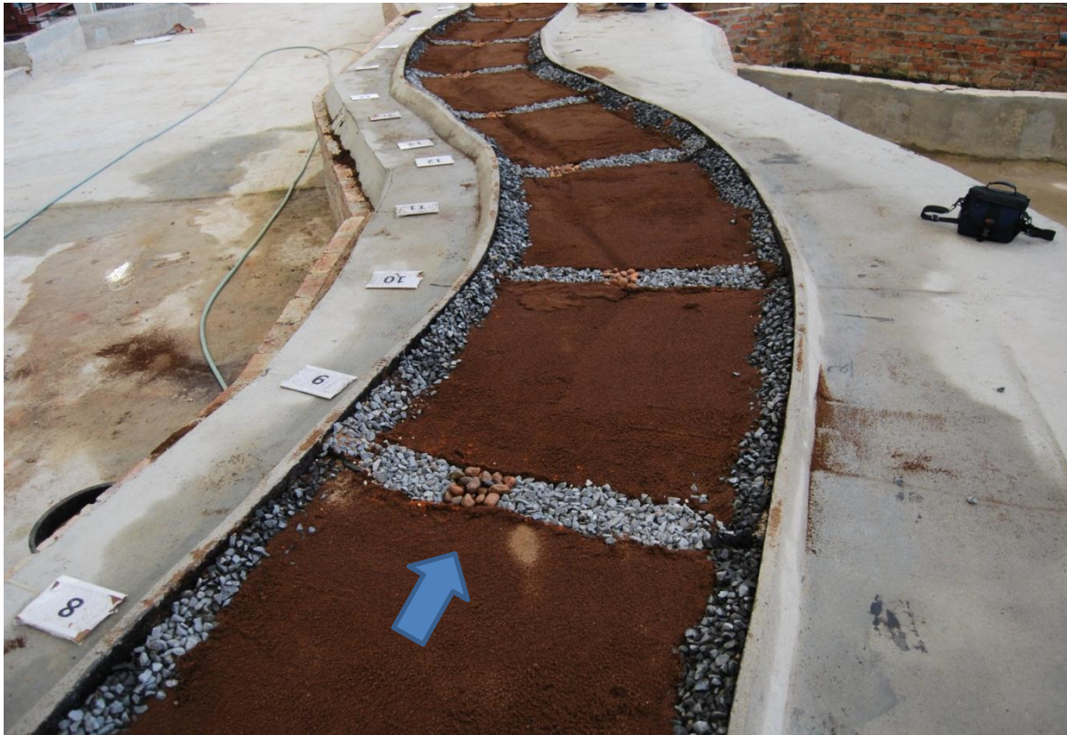
Figure 2-1: Typical riprap arrestors in laboratory setup (Institute for Water and Environmental Engineering, 2012)
