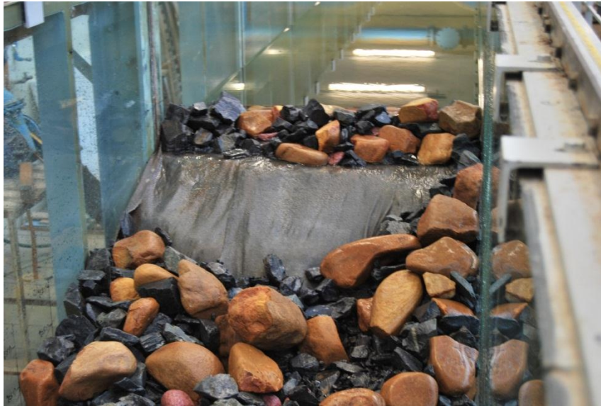
Figure 3-11: Example of failed arrestor structure, looking upstream (Test 131)
