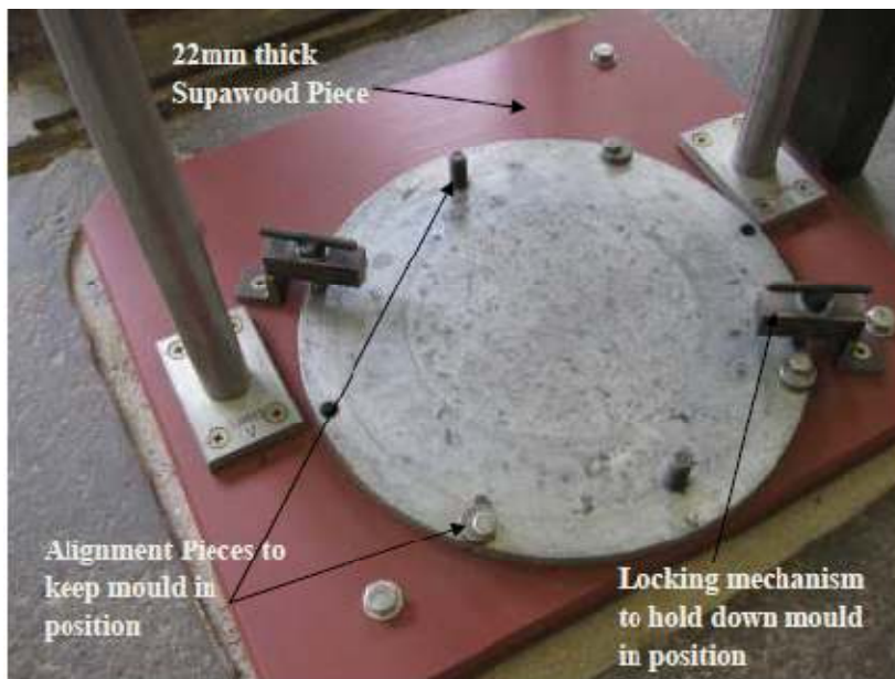
Plate 3-5: Bottom Wood Piece and Base Plate for holding mould in position
