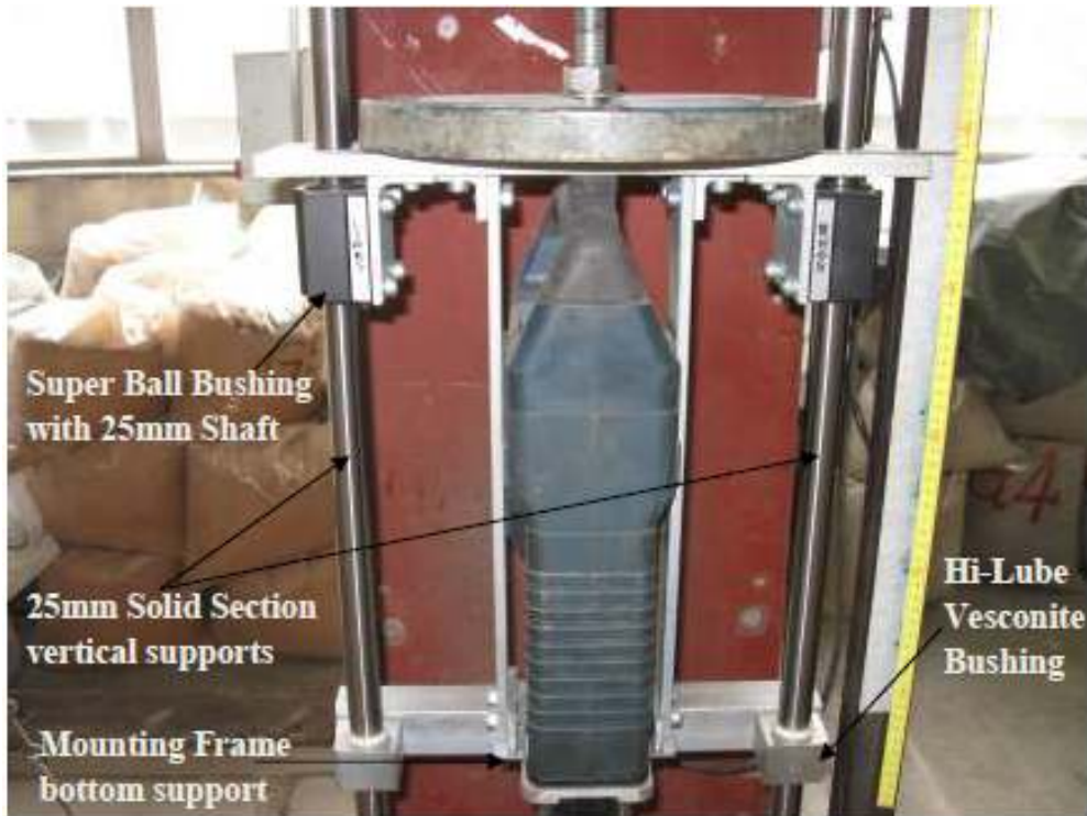
Plate 3-2: Vibratory Hammer Mounting Frame
