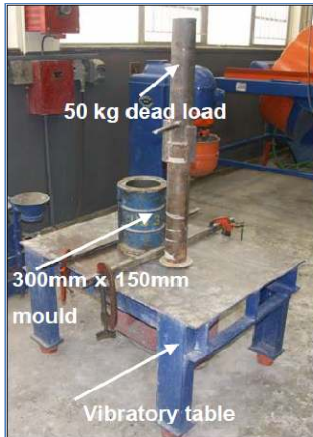
Plate 2-2: Stellenbosch University Vibratory Table Setup
