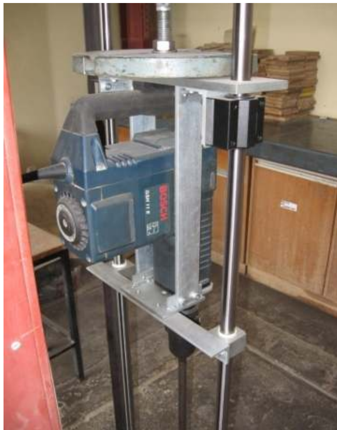
Plate 3-3: Rear view of Vibratory Hammer Mounting Frame
