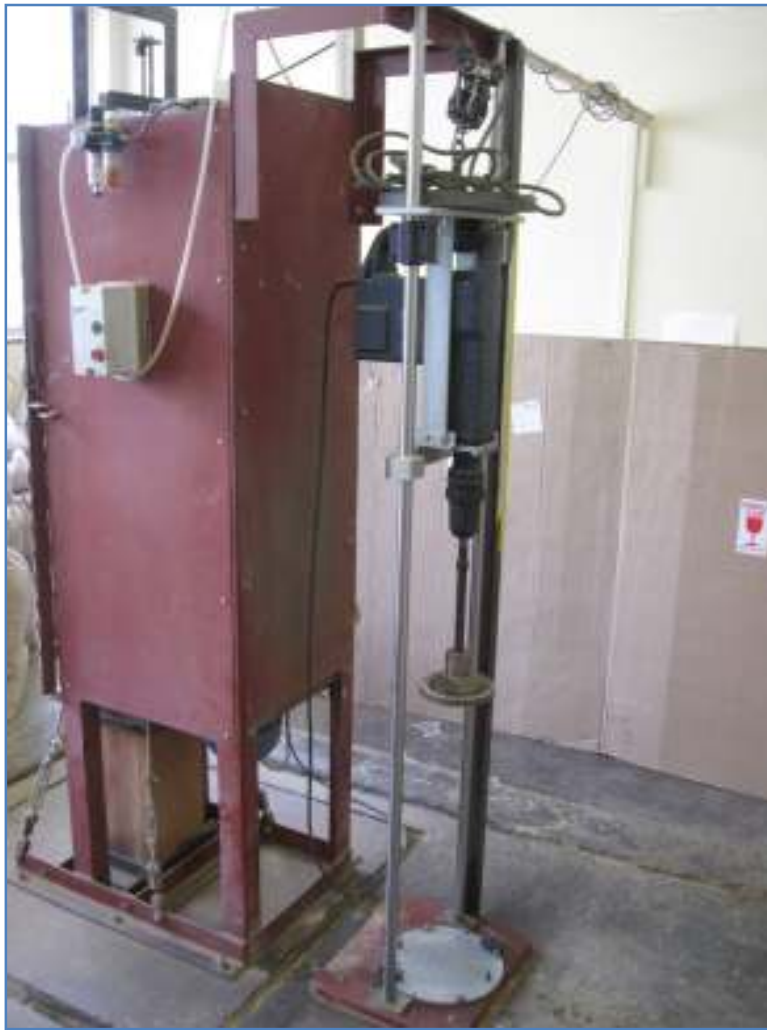
Plate 3-1: Stellenbosch University Setup of Upgraded Vibratory Hammer
