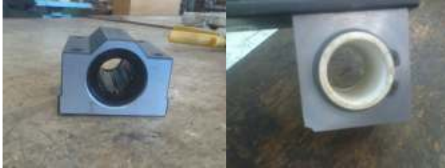
Plate 3-4: Super Ball Bushing and Hi-Lube Vesconite Bushing
