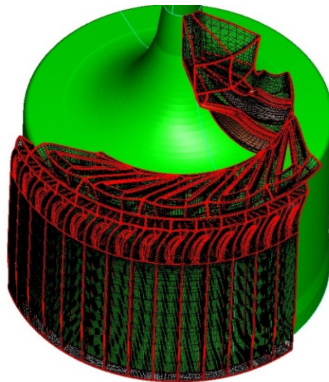
Figure D.5: Screenshot of the combined compressor mesh in AutoGrid5™ with a coarse (222) grid level
