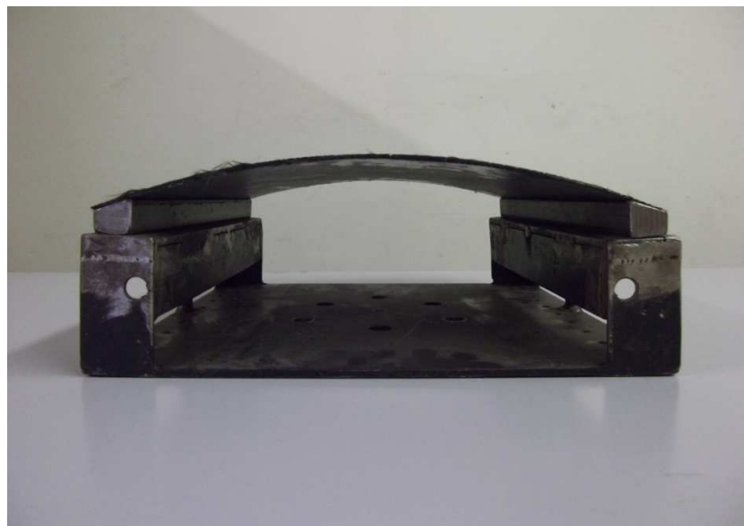
Figure 54 Adapted support assembly for curved laminate
