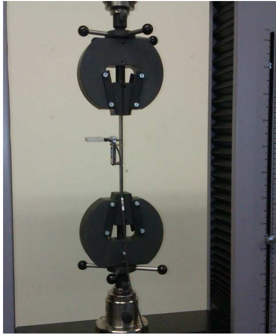
Figure 42 Tensile test setup
