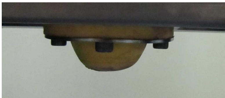
Figure 10 Rubber tip below trolley centrally mounted
