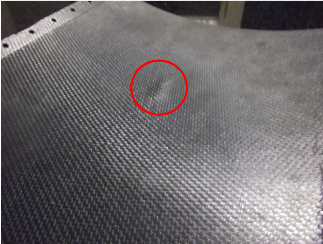
Figure 65 Damage on curved laminate. Picture taken from the underside of the panel. Note damage at clamping region and delamination area as indicated.
