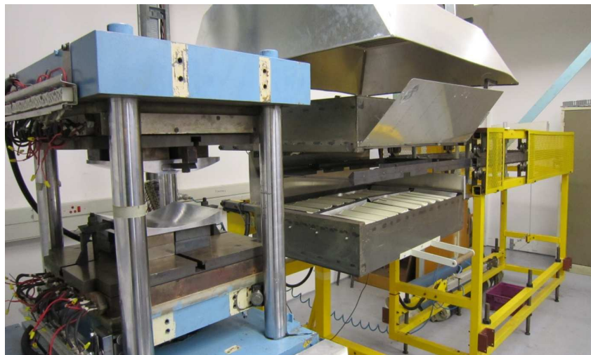
Figure 19 IR heater and press over view
