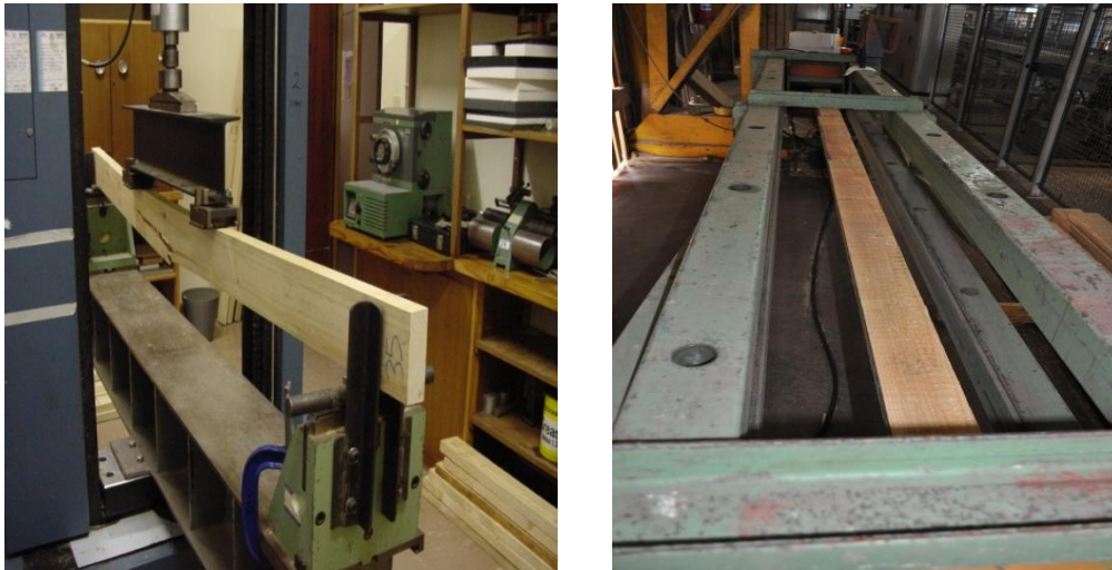
Figure 10: The bending test setup (left) and tension// test machine setup (right).
