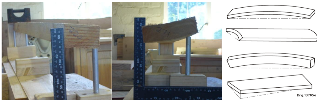
Figure 13: The jig used to measure warp (left and centre) and drawings of bow, cup, spring and twist (right).
