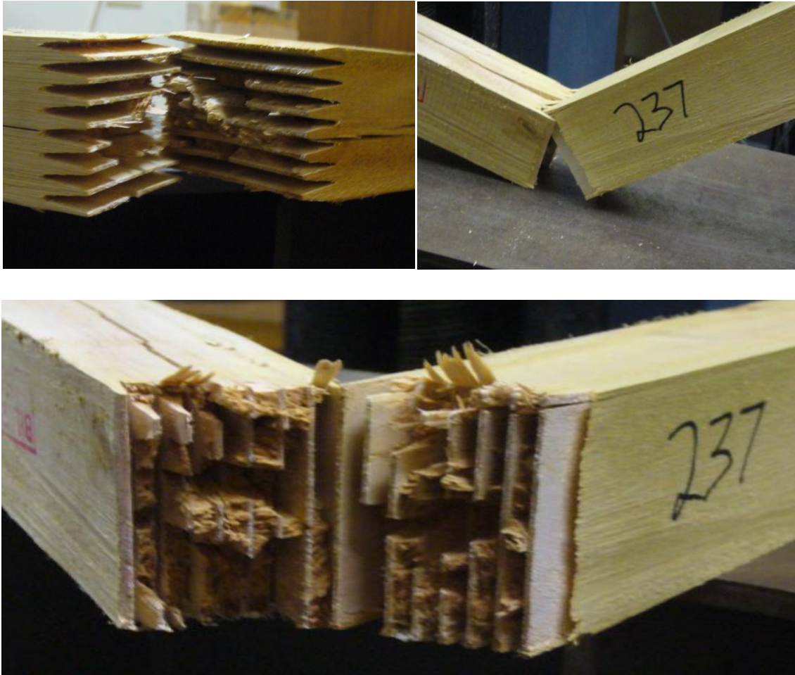
Figure 20: The failure modes of wet (top left) and dry young E. grandis 48 x 73 mm bending specimens.
