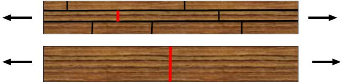
*Figure 5: Weak joint strength (thick line) occurrence in glulam (top) and finger-jointed boards (bottom) under load. Finger-jointed boards require adhesives with very good joint strength, whereas glulam consisting of multiple smaller wood pieces require adhesives with a lower creep tendency for optimal performance in service.
