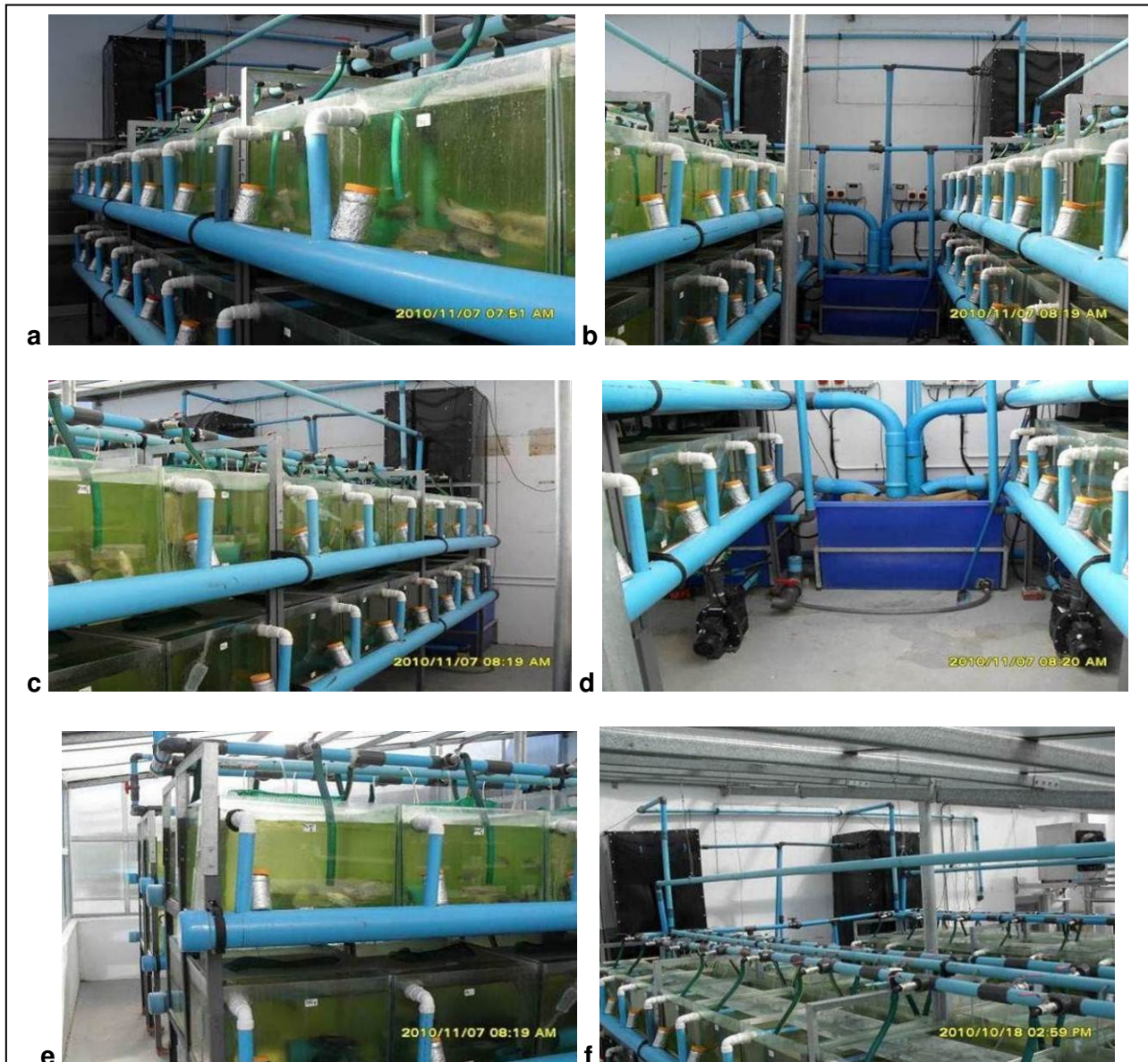
Plate 3.1 The recirculating aquaria system used during the study, incorporating 72-Glass Tanks showing:
