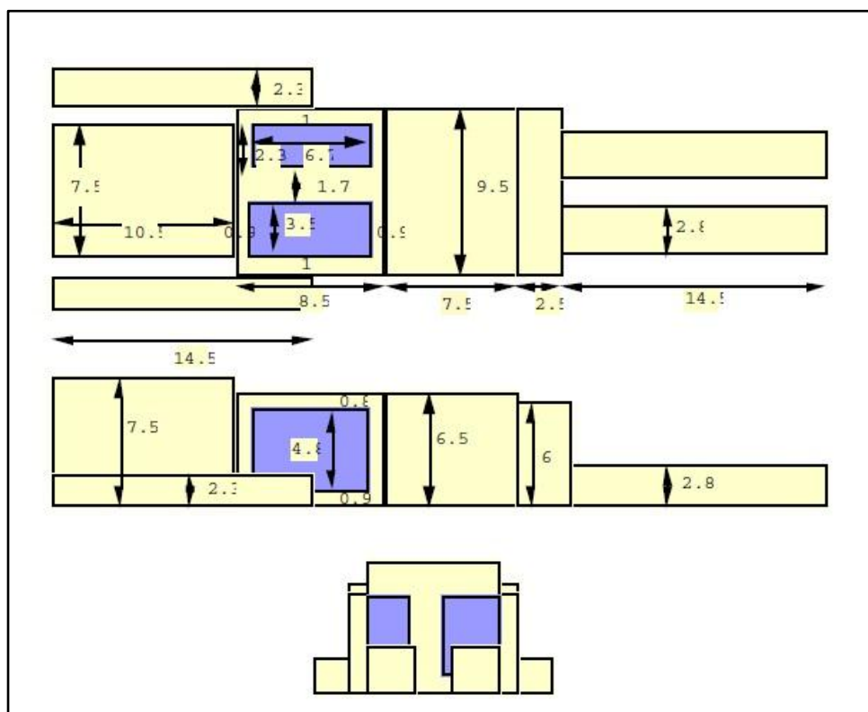
Figure 2.9: Neonatal simulation phantom. 29
