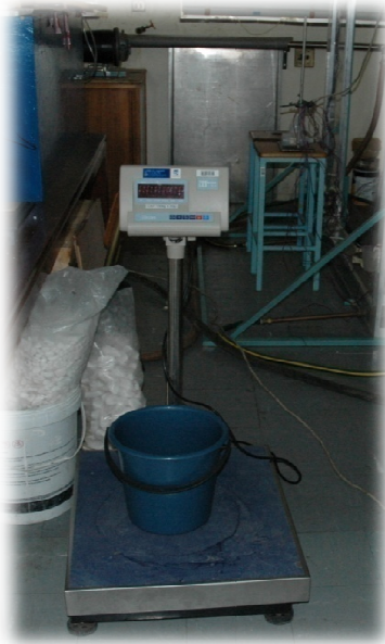
Figure 4.4: Scale and bucket used to check water mass flow
