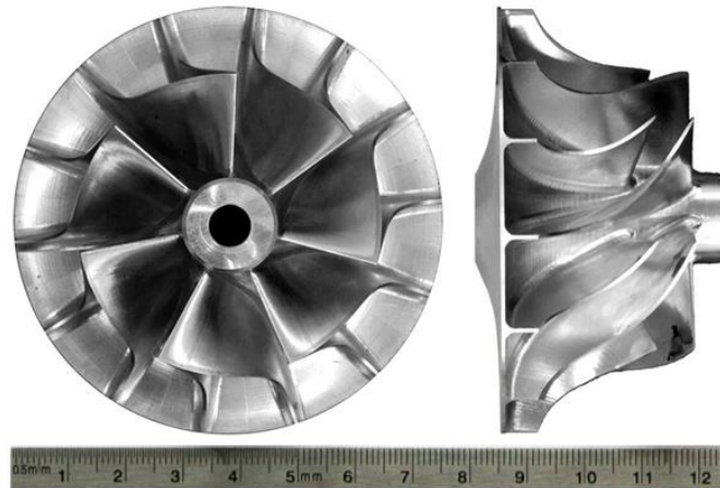
Figure 5.12: CNC milled impeller. Ruler units in cm.
