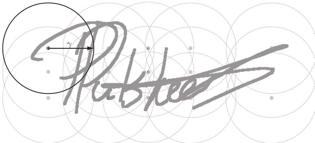
Figure 3.8: A signature image showing the location of fifteen retinas with radii \gamma . Each circular retina is centred on a centroid defined in the zoning process.
