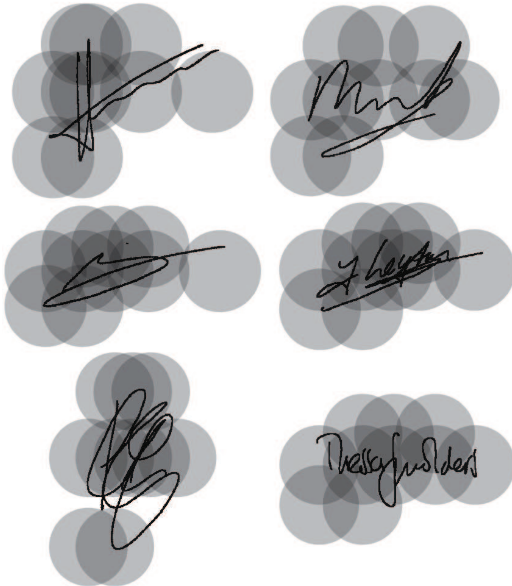
Figure 10.8: Local retinas that form part of the optimal ensemble \{2, 3, 4, 5, 6, 7, 8, 10, 11, 14, 16\} superimposed onto several signatures associated with different writers. The global retina (retina 16) is not shown.
