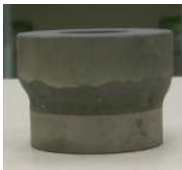
Figure 25 Green specimen of the sample shape from powder titanium
