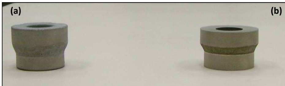
Figure 26 Shapes of samples before machining, (a) sample C, (b) sample D
