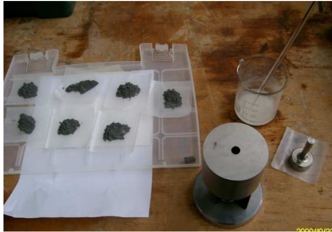
Figure 13 Right cylinder sample preparations before compaction showing the preweighed powder (left), lower punch and die assembly (middle, bottom), die wall lubrication solution (middle, top) and upper punch (right).
