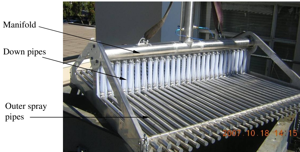
Figure 5-1: Spray frame designed for water distribution.
