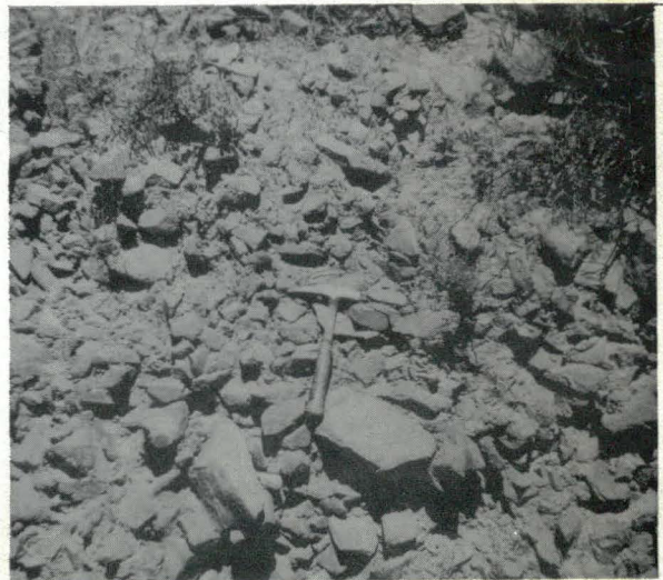
(f) Talus. Note angular cobbles as opposed to rounded river gravels in (d).
