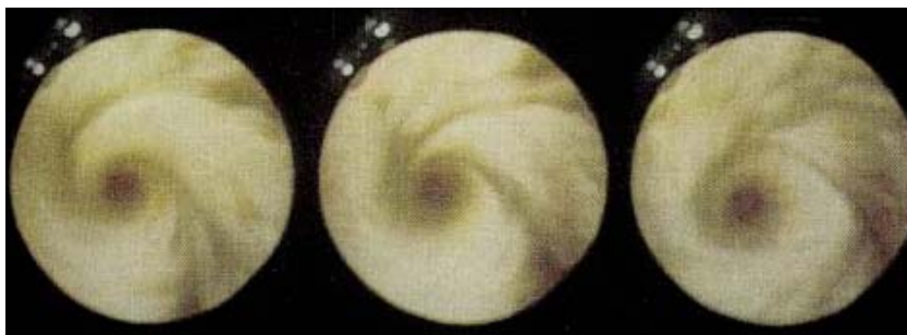
Figure 1.4: Vortices in SRM Window Tests [Sotter and Flandro (181)]
