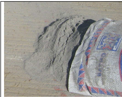
Figure 16: Pre-batched cementitious materials + sand + Polypropylene fibres
