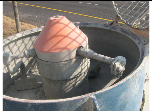
Figure 15: inside of mixer pan
