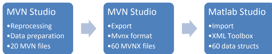
Figure 45: Flow of measurement data from MVN Studio into Matlab
