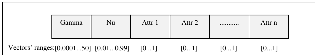
Figure 6.2: The agent encoding of the combined continuous and binary PSO as used in Geo-ND for simultaneous free parameter tuning and attribute subset selection
