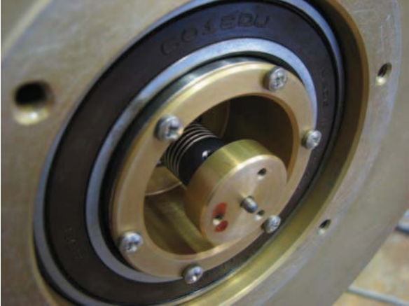
(b) Resolver installed
