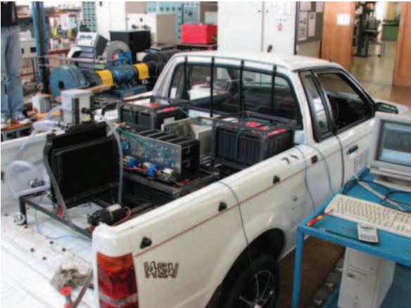
(d) Laboratory setup is moved to the test vehicle
