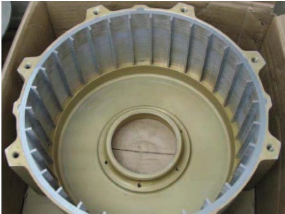
(c) Finished fitting the rotor laminations
