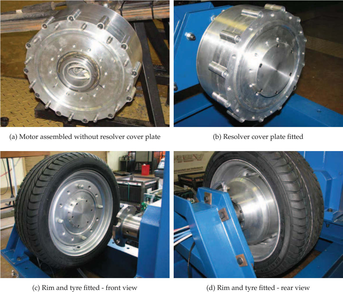
Figure 7.6: Assembled hub motor 1 ready for testing.
