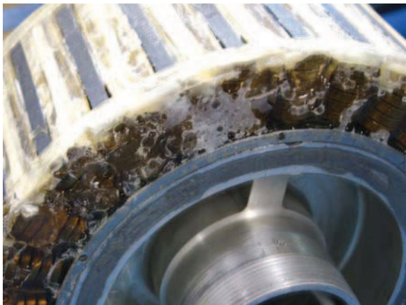
(e) Windings is completely covered by epoxy
