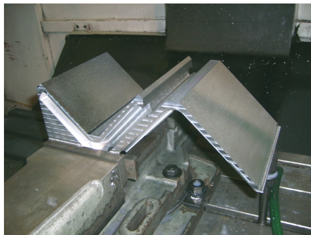
Figure 7: Milling of L-shaped mould
