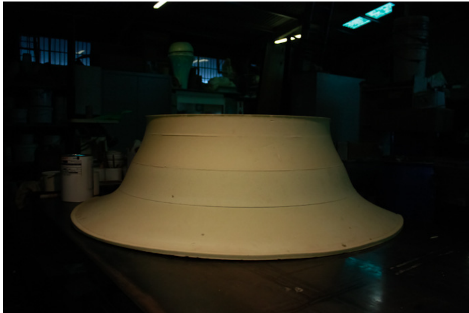
Figure 7.2: Polyurethane foam mould for diffuser.
