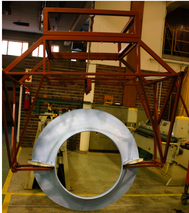
Figure 7.3: Manufactured support structure with diffuser.
