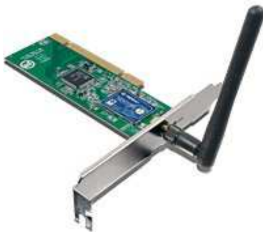
Figure 3.5: Wireless 802.11 transceiver. Reproduced from [4].
