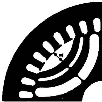
Fig. 4.3. Stator and rotor structure of the RSM designed for maximum torque/kVA (machine 4, Table 4.6)
