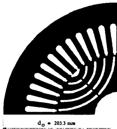
Fig. 4.4. Stator (48 slots) and rotor structure of the RSM designed for maximum torque (machine 6, Table 4.6)
