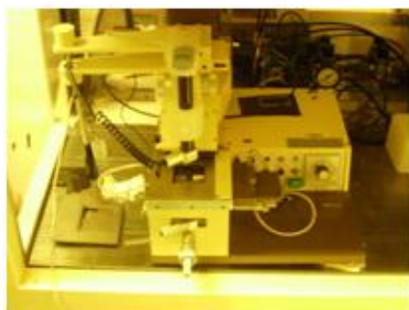
Figure 6.14: Picture of the lithography system.
