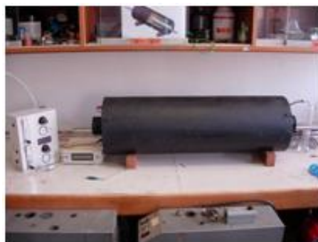
Figure 6.6: Picture of the tube furnace used for VLS growth. On the left are the gas bottles (out of sight) with the valve box just in picture. The furnace is the black object in the centre. Between the furnace and the valve box is the controller box.
