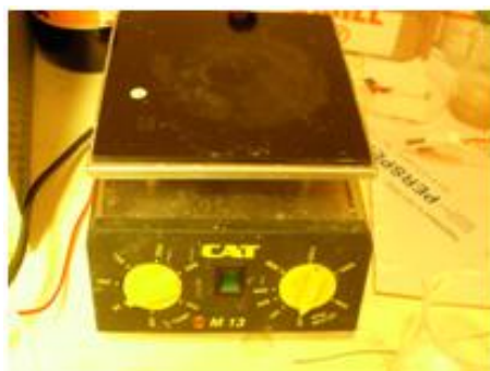
Figure 6.15: Picture of the mixer. A flask with chemicals in it is placed on top and a small white magnet is placed inside. The dials are then turned to spin the magnet and heat up the flask.
