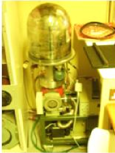
Figure 6.16: Picture of the thermal evaporator. The sample is loaded into the glass dome with the source material. The system is then put under vacuum to achieve the thermal evaporation.
