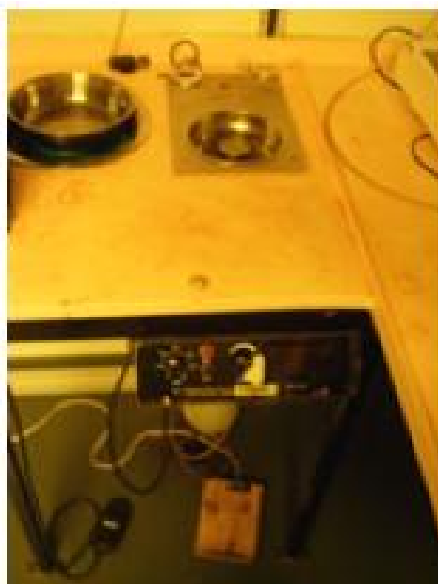
Figure 6.9: Picture of the spin table. At the back, the silver area is the spinning area. The black box connected to the table is the control box, used to set the speed. On the floor, the black pedals are to start and stop the spinner.
