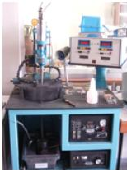
Figure 6.17: Picture of the Sonic Mill. To the left is the bit, at the top right is a motor used to position the bit. Bottom left is a bucket with the slurry. Bottom right are the two controller boxes for the system.
