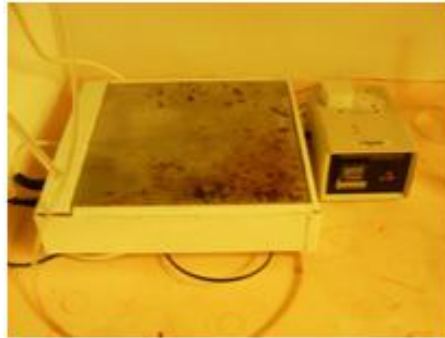
Figure 6.11: Picture of the hotplate. On the left is the hotplate itself and on the right the controller box.
